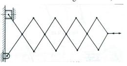
Q.31 Fig.shows schematic of a mechanism. Redraw the free-hand sketch on the answer book. Find out the total number of a kinematic links and number of kinematic pairs. Hence find out the degree of freedom for the mechanism.
