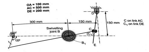
Q.9 Below fig. shows a mechanism in which crank OA is rotating anticlockwise at 20 rad/s.Link CD is in the form of rod sliding tangentially on an inverted and grounded semi-cylinder as shown, find out the linear velocity of slider E using graphical method of velocity polygon at the instant shown.
