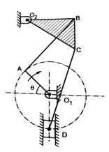
Q.15 Fig. shows a mechanism in which crank OA is rotating clockwise at 240 rpm. At the instant shown. Locate all ICRs for the mechanism and find out the velocity of slider E as well as the angular velocity of link BC using ICR method.
