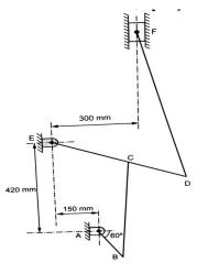
Q.11 Crank OA of a compound slider crank mechanism, as shown in fig. rotates at 20 r.p.m. Anticlockwise and gives motion to sliding blocks B & D. The dimensions of various links are OA = 300 mm, AB = 1200 mm, BC = 450 mm and CD = 450 mm. Determine the linear acceleration of block D.
