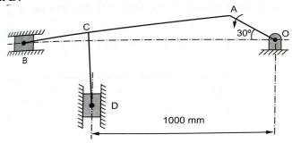
Q.12 Fig. shows the mechanism in which crank OA is rotating anticlockwise at 20 rad/s. At the 12 instant shown, find out the velocity and acceleration of slider B & D as well as the angular acceleration of link AB using relative method. (Use scale 1mm = 10 mm/s for the velocity polygon and  $1 \text{mm} = 200 \text{ mm/s}^2$  for acceleration polygon).
