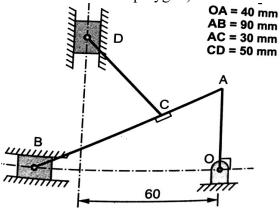
Q.13 The length of various links of a mechanism as shown in fig. are OA = 0.3m, AB = 1m, CD = 12 0.8m, and AC = CB. Determine for the given configuration, i) Velocity of slider D, ii) Velocity of slider B, iii) Angular velocity of CD, iv) Angular velocity of AB. If OA rotates at 60 r.p.m. clockwise use instataneous centre method. Also find absolute velocity of point C.
