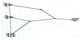
Q.29 Below Fig. shows schematic of a mechanism. Redraw the free-hand sketch on the answer book. Find out the total number of a kinematic links and number of kinematic pairs. Hence find out the degree of freedom for the mechanism.
